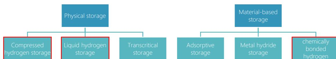
Figure 3: Storage methods for hydrogen
