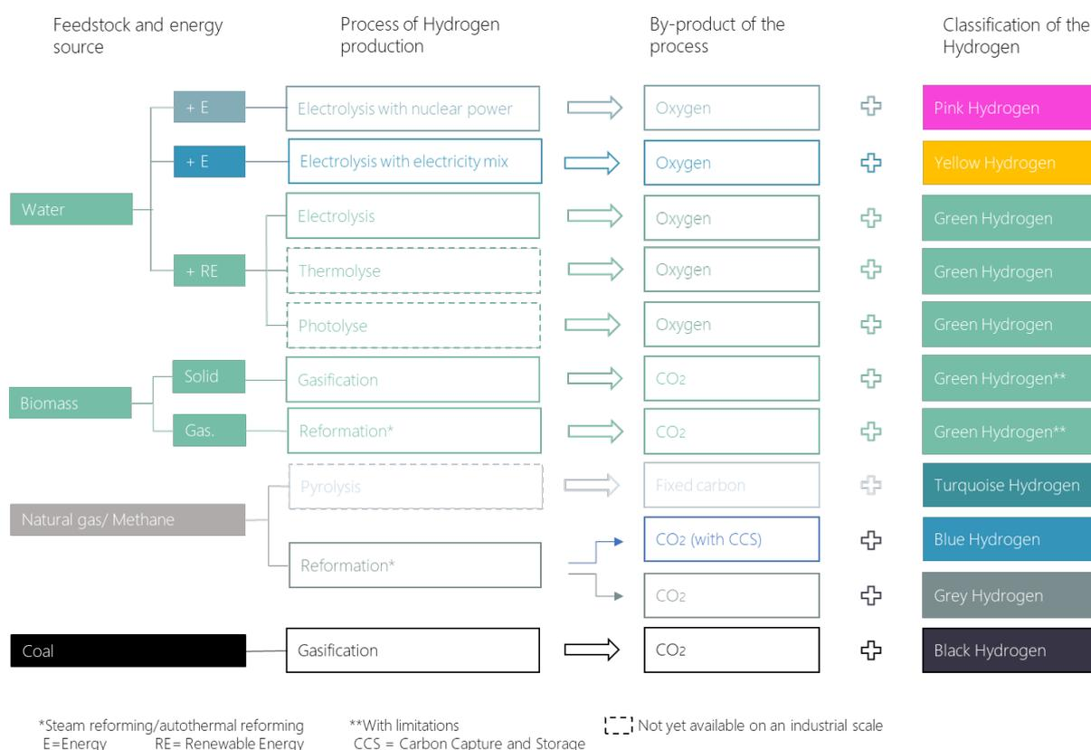
Figure 2: Production of hydrogen and colour coding (German Advisory Council on the Environment 2021)
