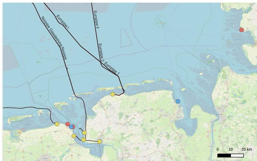
Figure 14: Pipelines in the North Sea, blue dots represent landing points for LNG, red dots represent landing points for electricity, yellow dots represent landing points for gas (own representation)
