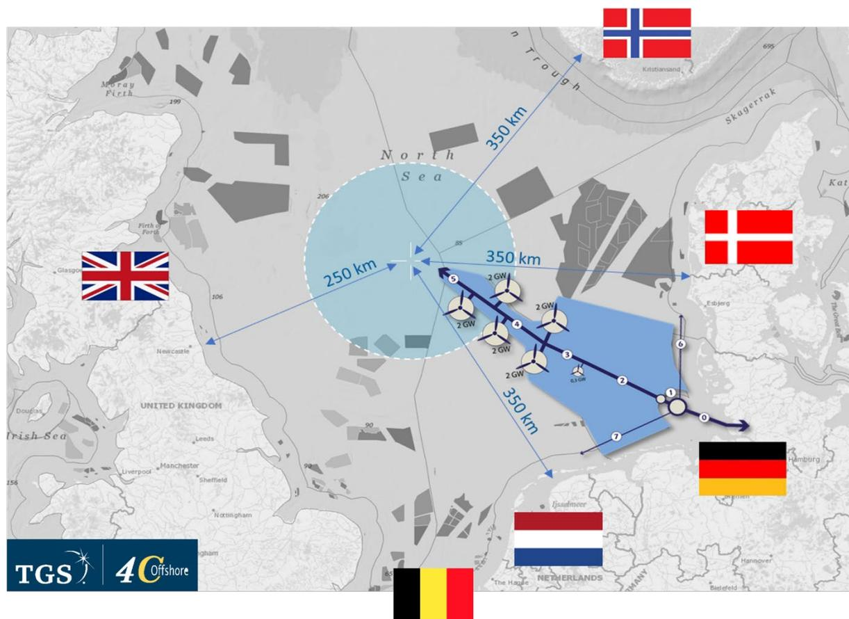
Figure 15: Representation of the planned hydrogen infrastructure in the North Sea (AquaVentus plans in blue, schematic course of a possible pipeline in dark blue) ©4cOffshore
