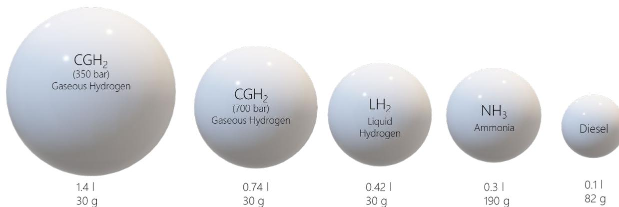
Figure 1: Volumetric and gravimetric energy density of fuels (drop sizes with fixed energy content of 1 kWh)
