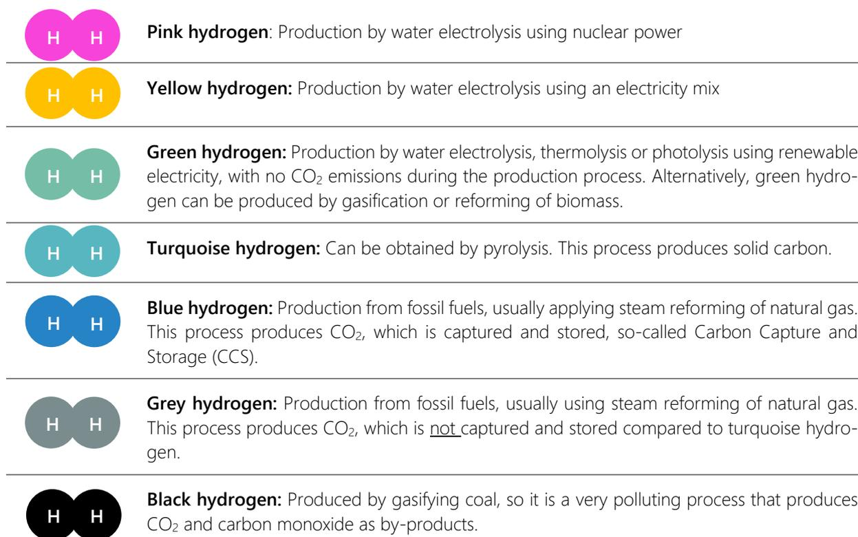
The Figure 2 provides a detailed overview of the aforementioned processes for the production of hydrogen with information on the feedstocks and energy sources, the by-products of the process and the resulting colour coding of the hydrogen.
