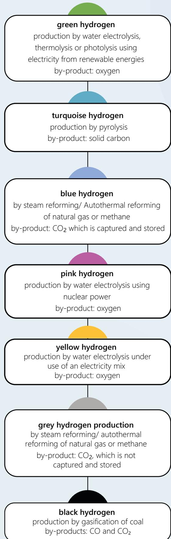
Figure 1: Production of hydrogen and colour coding; CO = carbon monoxide, CO<sub>2</sub> = carbon dioxide
